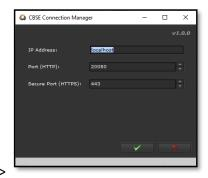
Connect to the evolution by changing the IP Address to "localhost" and change the default port to 20080, then accept by clicking on the tick
