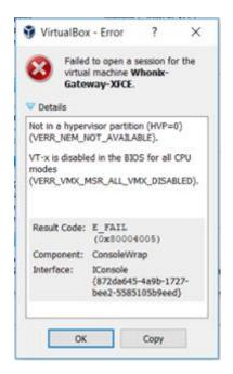
Should this message appear "Not in a hypervisor partition (HVP=0) (VERR\_NEM\_NOT\_AVAILABLE).VT-x is disabled in the BIOS for all CPU modes (VERR\_VMX\_MSR\_ALL\_VMX\_DISABLED)" then you must enable the AMD-V or Hyper-V function in the BIOS of your PC.
