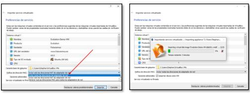
The only important thing is to leave the MAC as it is. **THE MAC ADDRESS MAY NOT BE CHANGED**. The consequence of changing it will cause a damaged VM which cannot be used anymore. So, **don't** select the option "Generate new MAC addresses...".
